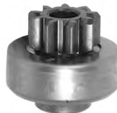
SND5039 Drive For Sea Doo PWC CCW; 9-Tooth; 6-Spline; For Denso Starters PIC 6190-2975; Gear OD 29mm Gear ID 12mm OAL 33.6mm Used on Sea-Doo Models 580, 650, 720 & XP757 REPL.: DENSO 028300-6000, 028300-7711; SEA DOO 295-500-089
