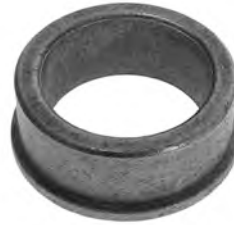
SMU7101 Bushing, Center Support For Mitsuba Starters PIC 6-23001; ID 15.95mm; OD 22.95mm; OAL 8.5mm; Used on ATV, Motorcycle and PWC
