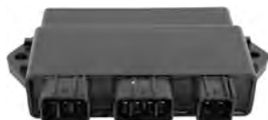
IYA6049 CDI Module For Yamaha Capacitive Discharge Ignition Used On 2004-08 Yamaha Grizzly YFM660F ATV REPL.: YAMAHA 5KM-85540-10-00
