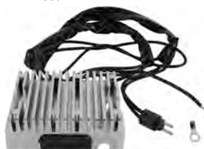
AHD6007-C Voltage Regulator / Rectifier For Harley Davidson M/C 12-Volt; Lead Length 38-51 Inches; 19A Systems; Shunt Type; Chrome Finish; For Black Finish, Use AHD6007 Used on Harley Davidson Sportster Models 1986-90 REPL.: HARLEY DAVIDSON 74523-84A; TRANSPO H2386C
