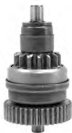
SMU5009 Drive CW; 14-Tooth; 40-Tooth Drive Gear; For Mitsuba Starters PIC 6191-2965; 14-Tooth is 28.42mm OD 40-Tooth is 46.5mm OD Drive is 72.36mm OAL Used in SCH0019 Starter Applications Also on Other ATVs and Scooters Made in China
