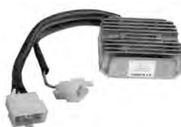
AYA6006 Voltage Regulator / Rectifier For Yamaha M/C PIC 8099-1502; 80mm L x 90mm W x 28mm H Hole Distance 67.5mm 3-Phase Field (+) Used on RD 350cc 1973-75 RD 400cc 1976-79 XS 650cc 1975-81 REPL.: YAMAHA 1A0-81970-60-00, 1L9-81910-50-00, 2G7-81910-50-00, 2L0-81910-50-00, 447-81970-10-00, 1L9-81970-60-00
