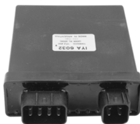
IYA6032 CDI Module For Yamaha Capacitive Discharge Ignition Used On YZF450, -SE 449cc 2006-09 REPL.: YAMAHA 5TG-85540-10-00
