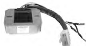
AHA6000 Voltage Regulator / Rectifier For Honda M/C PIC 8099-1316; 72mm L x 76mm W x 30mm H Hole Distance 60mm 3-Phase Field (+) Used on CB 750cc 1976
