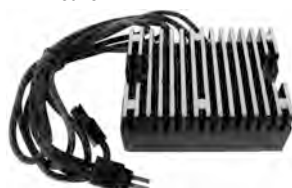
AHD6009 Voltage Regulator / Rectifier For Harley Davidson M/C 12-Volt; Lead Length 51 Inches; 32A Systems; Shunt Type; Black Finish; For Chrome Finish, Use AHD6009-C Used on Harley Davidson XL Models 1992-93 REPL.: HARLEY DAVIDSON 74523-92, 74523-92A; TRANSPO H2392
