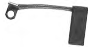
SMU7501 Brush For Mitsuba Starters PIC 5491-3004; 25mm L x 10mm W x 5mm H x 50mm LL; Used on Mitsuba Starters on ATV & Motorcycle Applications
