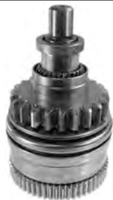
SMU5004 Drive For Arctic Cat CCW; 23-Tooth For Mitsuba Starters PIC 6191-2971; Gear 44.5mm OD Overall Length 107.2mm Used on Tigershark 770, 900, 1000, 1100 REPL.: ARCTCO 3008-408
