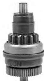
SMU5011 Drive For Honda CW; 14-Tooth; 54-Tooth Drive Gear; For Mitsuba Starters PIC 6191-2964; 14-Tooth is 27.84mm OD 54-Tooth is 34.2mm OD Drive is 74.24mm OAL Used in SMU0374 Starter Applications Also on Other ATVs and Scooters Made in China REPL.: HONDA 31209-GE1-714
