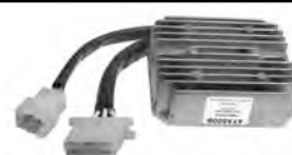
AYA6008 Voltage Regulator / Rectifier For Yamaha M/C PIC 8099-1504; 80mm L x 90mm W x 28mm H Hole Distance 67.5mm 3-Phase Field (-) Used on XS750 747cc 1978-79 XS850 826cc 1980-81 XS1100 1101cc 1978-81 REPL.: SHINDENGEN SH233; YAMAHA 1T4-81960-92-00, 1T4-81960-A0-00
