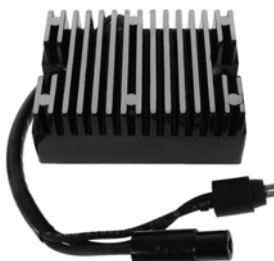
AHD6010 Voltage Regulator / Rectifier For Harley Davidson M/C 12-Volt; Lead Length 10 Inches; Shunt Type; Black Finish; For Chrome Finish, Use AHD6010-C Used on Harley Davidson Sportster Models 1994-03 REPL.: HARLEY DAVIDSON 74523-94; TRANSPO H2394
