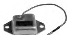
AYA6010 Voltage Regulator / Rectifier For Yamaha ATV, M/C Snowmobiles PIC 8099-1501, -1505; 48mm L x 72mm W x 16.6mm H Hole Distance 60mm Single Phase Used on BW200 Big Wheel 196cc 1985-86 Banshee YFZ350 347cc 1987-06 Blaster YFS200 195cc 1988-06 Bravo BR250 250cc 1982-87 EC540 1979-80 ET250 250cc 1978-81 ET300 295cc 1979-80 ET300 Enticer 295cc 1983-84 ET340 340cc 1978-80 ET340 Enticer 340cc 1982-87 ET340T Enticer 340cc 1982-87 EX340 340cc 1978 EX440 440cc 1978-81 Excel EC340 340cc 1981-83 Excel III EC340 340cc 1984-87 Also Fits Other Similar Applications REPL.: YAMAHA 82F-81910-00-00, 82F-81910-A0-00, 8H4-81910-50-00
