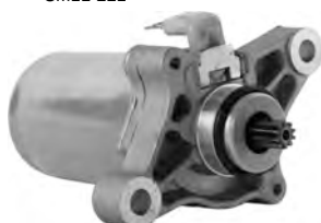
SCH0096 For Kymco, Sym, Others PMDD; 12-Volt; CCW; 10-Spline; Used On Kymco 50cc Engines REPL.: KYMCO 00104202, 31210-GAK-900
