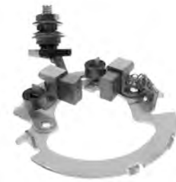
SMU1303 Brush Holder, w/Brushes For Honda PIC 5591-1303; 2-Brush Plate Both Brushes Included Also Includes Battery Stud and Hardware Used on Honda ATVs REPL.: HONDA 31206-KW1-901
