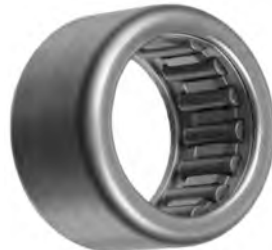
SMU7002 Bearing, Needle For Mitsubishi, Mitsuba Starters PIC 4-2014; ID 14.3mm; OD 20.0mm; OAL 11.9mm; Used on Mitsubishi OSGR Starters (CS Frame), Mitsuba Motorcycle / ATV Starters REPL.: REFERENCE NUMBER HK-1412
