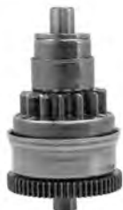
SMU5006 Drive CW; 14-Tooth; 61-Tooth Drive Gear; For Mitsuba Starters PIC 6191-2967; 14-Tooth is 27.78mm OD 61-Tooth is 37.52mm OD Drive is 67.54mm OAL Used on 50cc ATVs and Scooters Made in China
