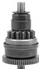
SMU5012 Drive For Honda CW; 14-Tooth; 63-Tooth Drive Gear; For Mitsuba Starters PIC 6191-2966; 14-Tooth is 27.75mm OD 63-Tooth is 39.3mm OD Drive is 70.38mm OAL Used in SCH0021 Starter Applications Also on Other and Scooters Made in China
