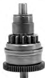
SMU5007 Drive CW; 14-Tooth; 62-Tooth Drive Gear; For Mitsuba Starters PIC 6191-2968; 14-Tooth is 27.60mm OD 62-Tooth is 39.50mm OD Drive is 70.50mm OAL Used on 50cc ATVs and Scooters Made in China
