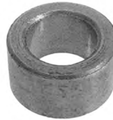
SMU7102 Bushing, C/E For Mitsuba Starters PIC 6-14004; ID 8.9mm; OD 14.07mm; OAL 8mm; Used on ATV, Motorcycle and PWC
