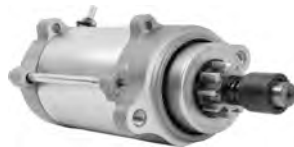
SND0734 For Ski-Doo Snowmobiles PMDD; 12-Volt; CW; 9-Tooth; PIC 190-6266; Used on
