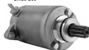
SCH0101 For Suzuki PMDD; 12-Volt; CCW; 9-Spline; Used on European Applications Used On 1995-00 Suzuki Burgman AN125, AN150 REPL.: DENSO 228000-3450; SUZUKI 31100-20E00
