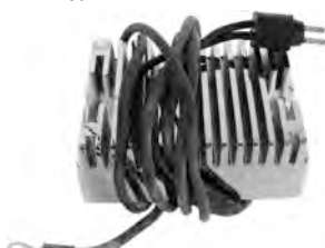
AHD6008-C Voltage Regulator / Rectifier For Harley Davidson M/C 12-Volt; Lead Length 51 Inches; 32A Systems; Shunt Type; Chrome Finish; For Black Finish, Use AHD6008 Used on Harley Davidson Sportster Models w/5-Speed 1991 REPL.: HARLEY DAVIDSON 74523-91; TRANSPO H2391C
