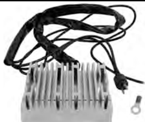
AHD6006-C Voltage Regulator / Rectifier For Harley Davidson M/C 12-Volt; Lead Length 51 Inches; Shunt Type; Chrome Finish; For Black Finish, Use AHD6006 Used on Harley Davidson Sportster Models 1984-85 REPL.: HARLEY DAVIDSON 74523-84; TRANSPO H2384C
