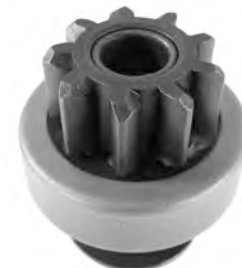
SND5057 Drive For Kawasaki CW; 9-Tooth; 5-Spline; For Denso Starters PIC 6190-2983; Gear OD 28.7mm Gear ID 11mm OAL 53.8mm Lester 18450, 18982; Used on Kawasaki Mule REPL.: DAIHATSU 28011-13060-000; DENSO 028300-5400; KAWASAKI 13081-2164; TOYOTA 28011-13060
