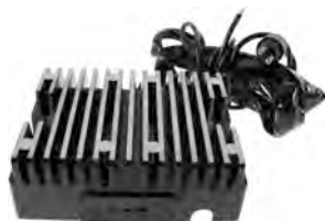
AHD6007 Voltage Regulator / Rectifier For Harley Davidson M/C PIC 8099-1911; 12-Volt; Lead Length 38-51 Inches; 19A Systems; Shunt Type; Black Finish; For Chrome Finish, Use AHD6007-C Used on Harley Davidson Sportster Models 1986-90 REPL.: HARLEY DAVIDSON 74523-84A; TRANSPO H2386
