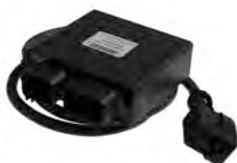
IHA6035 CDI Module For Honda Capacitive Discharge Ignition PIC 9900-5126A; 70mm L x 75.2mm W x 26mm H Hole Distance 86mm w/Multicurve Used On TRX450R Sportrax 433cc 2004-05 REPL.: HONDA 30410-HP1-003
