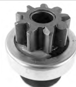
SND5056 Drive For Kawasaki, Kubota, John Deere CCW; 9-Tooth; 5-Spline; For Denso Starters PIC 6190-2986; Gear OD 29.1mm Gear ID 11mm OAL 53.6mm Lester 18010, 18011, 18012, 18404, 18512; Used on 1986-99 Kawasaki, Kubota, John Deere, Others REPL.: DENSO 028300-5720; JOHN DEERE AM105579; KAWASAKI 13081-2108
