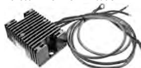
AHD6014 Voltage Regulator / Rectifier For Harley Davidson M/C 4-Wire 37mm L x 91mm W x 64.8mm H Hole Distance 82.5mm Single Phase w/Sensor Used on Harley Davidson Motorcycles
