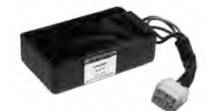
IK16000 CDI Module For Kawasaki Capacitive Discharge Ignition PIC 9900-5160; 55.5mm L x 93.5mm W x 24mm H w/DC-DC Advance Used On KLX110 80cc 2002-09 REPL.: KAWASAKI 21119-1612
