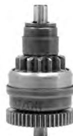
SMU5010 Drive CW; 14-Tooth 47-Tooth Drive Gear; For Mitsuba Starters PIC 6191-2963; 14-Tooth is 27.84mm OD 47-Tooth is 40.0mm OD Drive is 74.2mm OAL Used in SCH0012 Starter Applications Also on Other 100cc ATVs and Scooters Made in China
