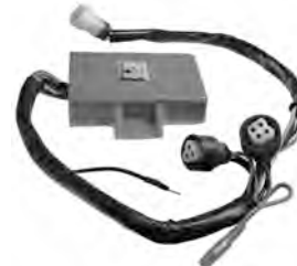
IYA6025 CDI Module For Yamaha Capacitive Discharge Ignition PIC 9900-5134; 98mm L x 70mm W x 26mm H Hole Distance 86mm w/Microcontroller w/Monocurve Multicurve Version is IYA6017 Used On YFM350X Warrior 348cc 1990-95 REPL.: YAMAHA 3GD-85540-20-00
