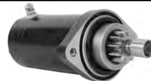
SHI0071 For Yamaha PWC DD; 12-Volt; CCW; 11-Tooth; LESTER 18303; PIC 104-169; 6K8 Engine Booth Mounting Holes Threaded Used on 1987-93 Yamaha WJ500, WR500 PWC REPL.: HITACHI S108-102, S108-102A, -2B; YAMAHA 6K8-81800-10-00, 6K8-81800-11-00, 6K8-81800-12-00
